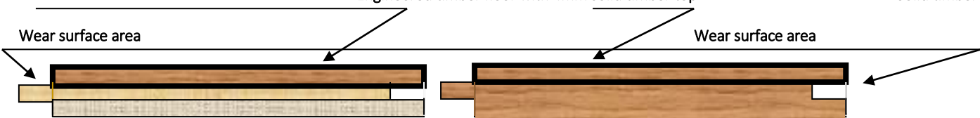
Engineered timber floor with 4mm solid timber top
